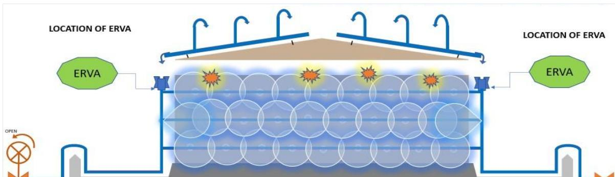
Animated picture showing Water Spray system post roof blow off condition.
