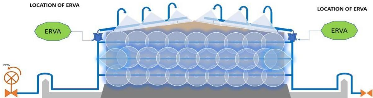
Above image of Spray system at Tank indicates Spray Nozzles at Tank shell, roof, and ERVA
